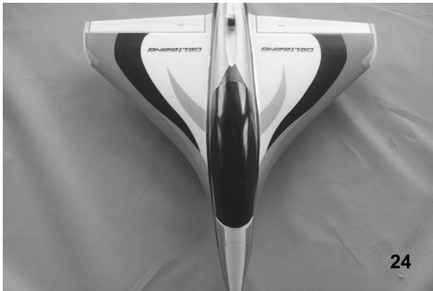
Fig. 24 - Install the canopy.
