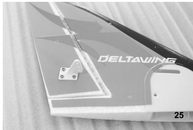
Fig. 25 - Install the control horn.
