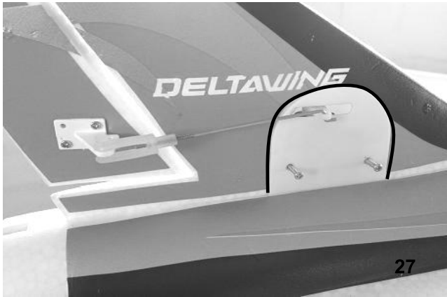
Fig. 27 - Connect the push rods to the servo arm and then to the control horn, then secure the servo fairing with screws. Caution! Rudder servo fairings are factory-installed, cutting off the decal along the slot can lift up servo fairing to replace the rudder servo.
