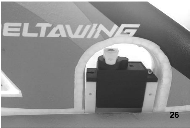
Fig. 26 - Apply glue to the slot of fuselage, and then install the Vertical Stabilizer to it. Hold it in position until the glue fully secured.
