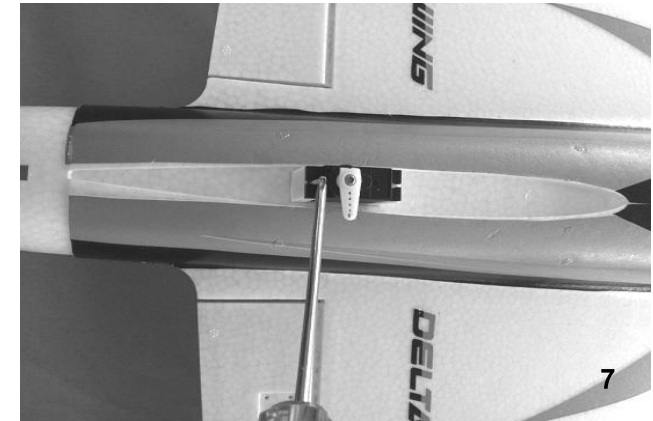
Fig. 7 - Secure the rudder servo with screws.
