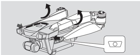
After releasing the arm buttons, the buttons are fully popped up, indicating that the arms are fully unfolded
