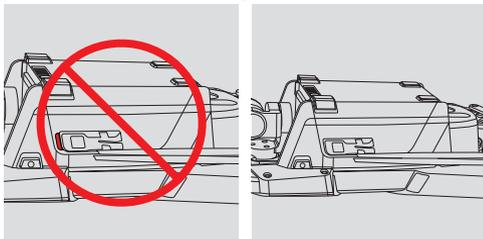
Make sure the red labels under the battery buckles are not visible to ensure the battery is securely installed
