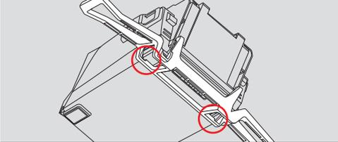
1 Wrap the landing gear over the both sides of the battery footpads
