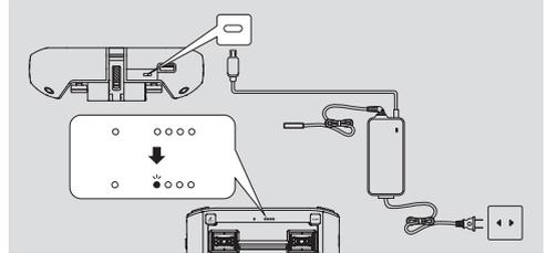
Plug the charging cable into the USB-C Port. It takes about 2.5 hours to fully charge.
