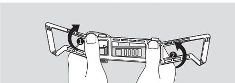
1 Hold one side of the landing gear and push in the direction shown to remove it from the battery footpad
