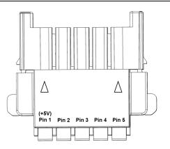
3. Connect the signal cable according to pin definition (2.2.6.1) and must connect to the Pin 1 (+5V).
