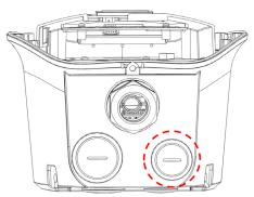
2. Remove the water proof cap and pass through the signal cable with appropriate conduit or cable gland.
