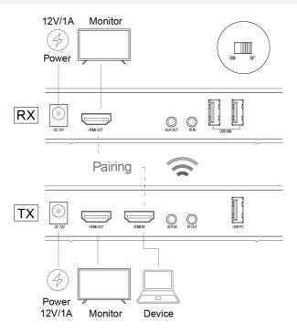
When the monitor is connected to the receiver, and there is no signal, ensure the transmitter and receiver are set to Splitter mode (SP). Disconnect the receiver and transmitter from the power adapter. Reconnect the transmitter and then the receiver to the power adapter.
