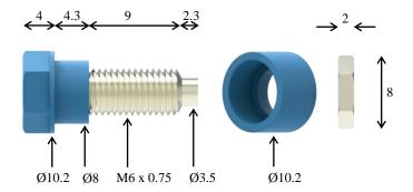
Thanks to the nut, the socket can be removed from the panel to be replaced or re-used.
