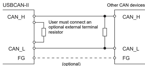
1. (If you use your own resistors) Connect the resistors as shown in the diagram.
