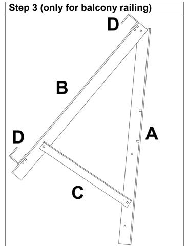
Use part C and insert it into the hole of B and the middle hole of A to mount the bracket for the 35° angle. Secure part C with two M8 hex nuts. Tighten the nuts with a 13 mm wrench.
