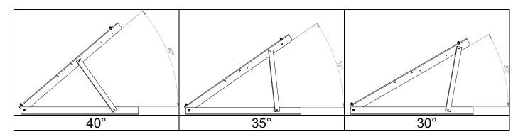
By loosening and adjusting the screw inserted in the rail, you can change the angle of the bracket. **Technical specifications**
