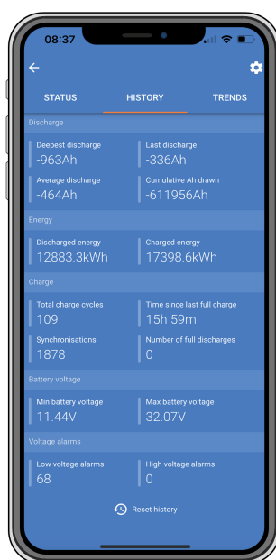
VictronConnect app showing battery monitor history
