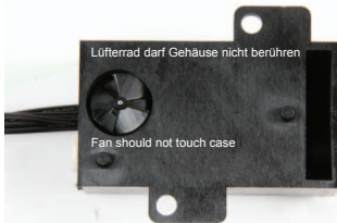
Abbildung 6: Wechsel Heizelement Figure 6: Replacing the Heating Element
