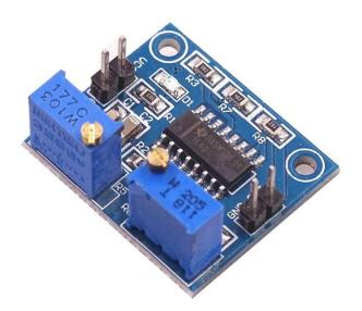
TL494 device integrates all the functions required to build a pulse width modulation (PWM) control circuit on a single chip. The device is mainly designed for power control, which provides flexibility to customize the specific application of power control circuit.
