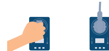
Figure 3 Plugging the device into universal temperature switch
