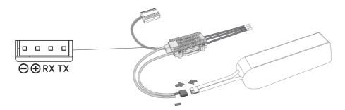
3.2 If the ESC do not have individual programming interface, then the pin is needed, according to the connection diagram as shown below, connect the ESC signal cable with the Bluetooth module cable. A special pins should be needed when connecting both of them, pay attention to the same colour cable should be connected correspondingly, and then connect the ESC to the battery.
