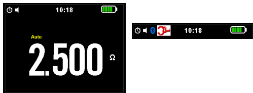
Figure 3: Ground resistance measurement
