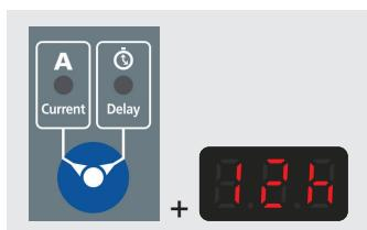
Press the «Current/Delay» button . The Delay LED will light up.
