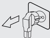
Disconnect the device from the power supply.
