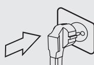
The cable automatically detects the type of socket to which it is connected, and regulates the current accordingly.
