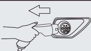
When the vehicle is fully charged, the charger will show
