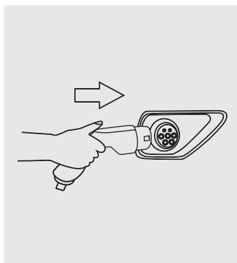
Once the appropriate charge setting has been selected, connect the device to the vehicle. The charger shows on the display (connected).
