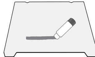
③ When the first layer of the model is not glued, it is recommended to apply glue stick evenly on the surface of the platform. The residual solid glue left after the printing can be cleaned with clean water.
