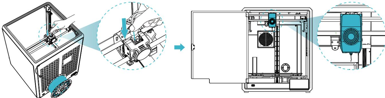
⑧ Lock the extrusion switch. ⑨ Restore the PTFE tube to its original position.
