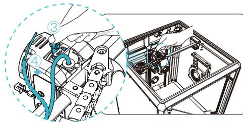
⑤ Completely remove the filament from the PTFE tube.
