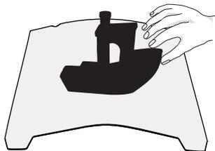
① Together with the flexible platform after the printed model has been cooled down Remove from the device and partially bend the platform slightly to separate the model from the platform.(No excessive bending of the platform to prevent it from being deformed and unusable)
