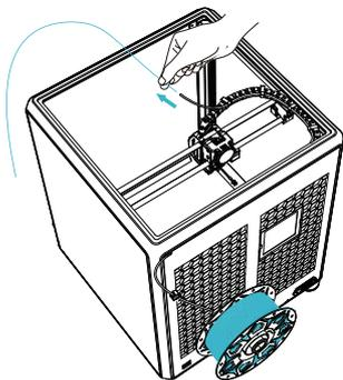
⑥ Insert the filament from the outside until it comes out of the other end of the PTFE tube.
