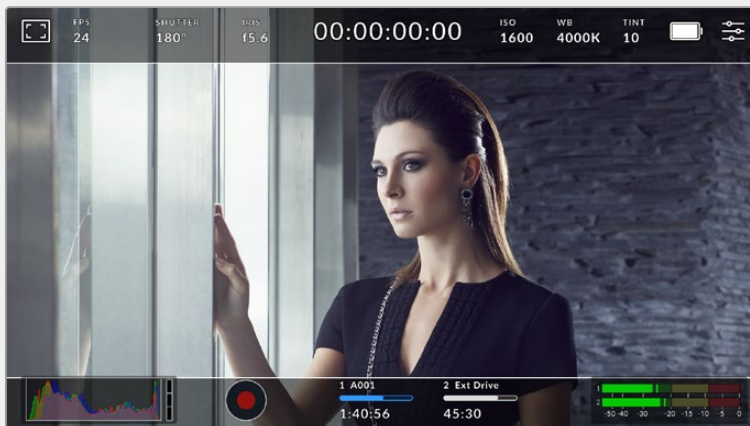
The LCD touchscreen with 2.40:1 frame guides enabled
