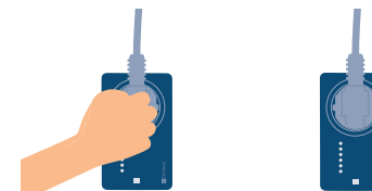
Figure 6 Plugging the device into the water protection switch
