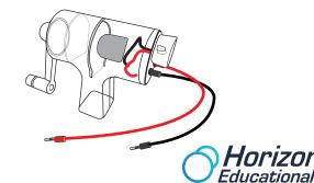
c. Connect the other end of the cable from the hand crank generator to the potentiometer. Ensure to respect the color code.
