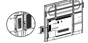
Secure the Navigator with one screw and two captive screws.
