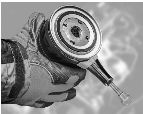
Figure 4: Unscrewing the oil filter
