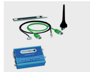
External modem for architecture with more than 10 EVlink Pro AC and/or EcoStruxure EV Charging Expert Manage wireless communication of large infrastructure and installation requiring load management. Modem reference: EVP3MM Antenna reference: EVP2MX
