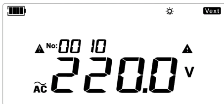
Figure 13.23 AC voltage measurement
