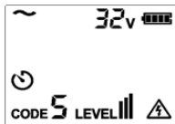
Figure 12.1f AC voltage (>30V) measurement
