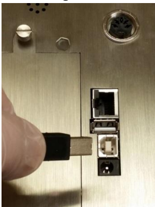
Connecting USB - B Client
