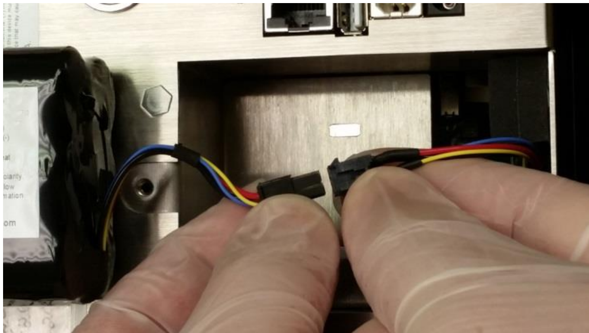
Step 3 – Insert battery connector plug into matching socket on matching wired connector in the battery compartment.
