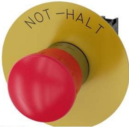
EM. STOP MUSHROOM PUSHBUTTON, 22MM, ROUND, METAL, SHINY, RED, 40MM, LATCHING, ROTATE TO UNLATCH, WITH YELLOW BACKING PLATE, INSCRIPTION: NOT-HALT, WITH HOLDER, 1NC, SCREW TERMINAL
