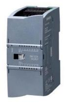
SIPLUS S7-1200 SM 1223 based on 6ES7223-1QH32-0XB0 mit Conformal Coating, -40...+70°C, start up -25°C, SIMATIC S7-1200, Digitalein-/ ausgabe SM 1223, 8 DI AC/8 DO RLY, 8 DI 120/230V AC, 8 DO Relais 2A
