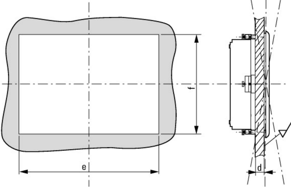
$1,5 \text{ mm} \leq d \leq 4 \text{ mm}$ ,  $e = 388 \text{ mm}$ ,  $f = 239 \text{ mm}$ ,  $\# = 10^\circ$
