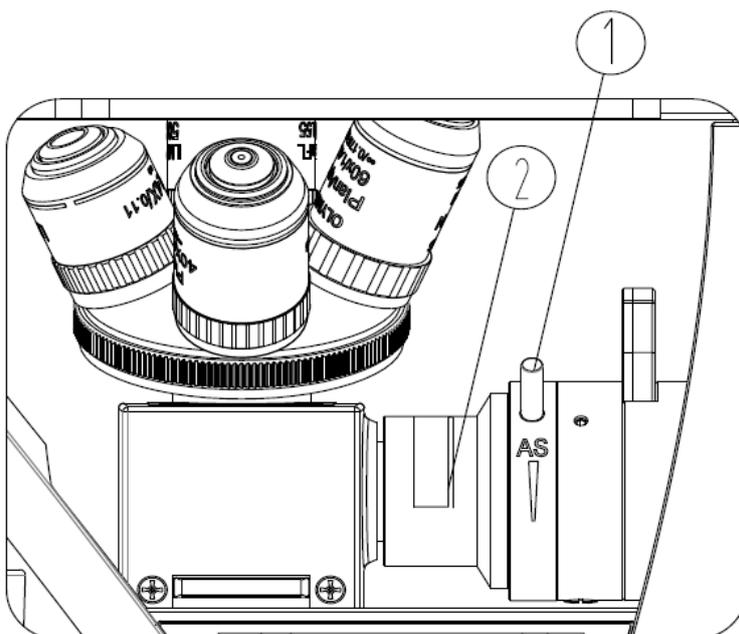
For the application of the polarization method, an analyser slide [3] and a polariser slide [1+2] are included in the scope of delivery, which must also be placed in the appropriate slots.
