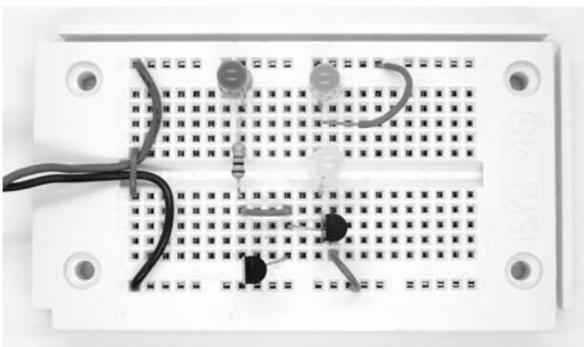
Fig. 27: Transistor as temperature sensor (Aufbau8.jpg)
