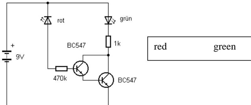
Fig. 22: Gain of the LED reverse current (Schaltung6.jpg)
