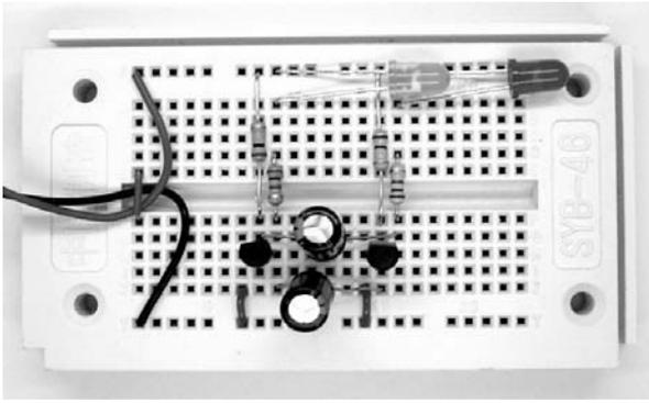
Fig. 33: A slow alternating flasher (F\_Blinker1.jpg)
