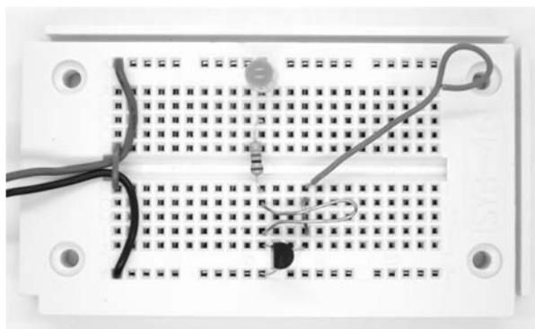
Fig. 43: Detection of electric charges (Aufbau16.jpg)
