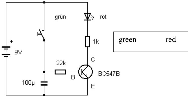
Fig. 16: Delayed switching-off (Schaltung3.jpg)
