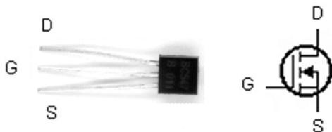
Fig. 9: The MOSFET transistor BS170 (B\_FET.jpg)
