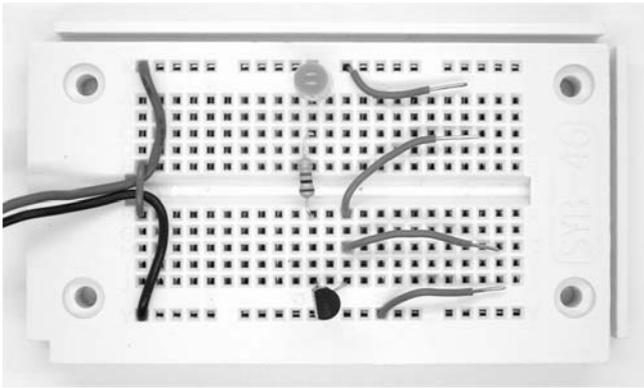
Fig. 39: Charging and discharging the gate (Aufbau14.jpg)
