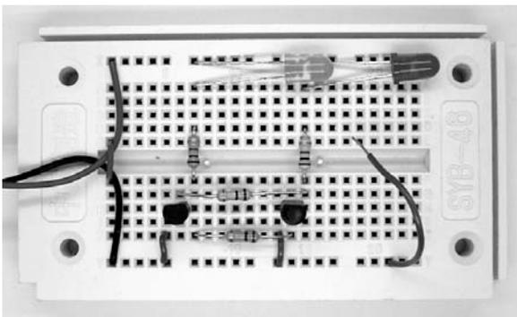
Fig. 29: The flip-flop (F\_Flipflop1.jpg)
