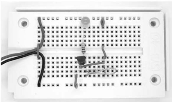
Fig. 47: The temperature sensor (Aufbau18.jpg)
