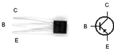
Fig. 8: The PNP transistor BC557 (B\_PNP.jpg)
