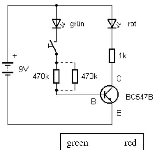
Fig. 12: An NPN transistor in the emitter circuit (Schaltung1.jpg)
