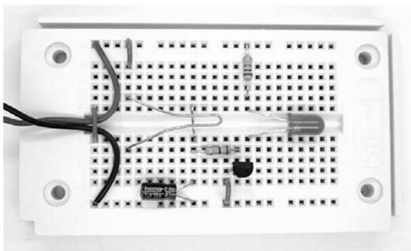
Fig. 17: The afterglow electric torch (F\_NPN3.jpg)
