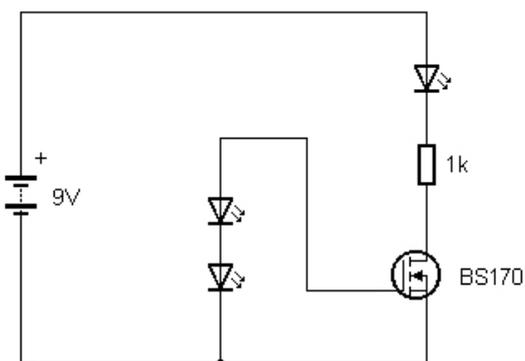
Fig. 44: LEDs as photovoltaic cells (Schaltung17.jpg)
