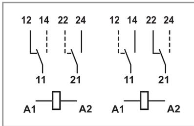
Alternative selection of NO and NC contacts to provide Forcibly guided (mechanically linked) contacts, in accordance with EN 50205 (type B).
