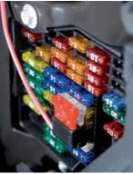
Step 1: To connect the wire terminal of Vehicle Fuse block extension to device and check the rating on device
