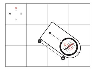
2. Turn the capsule until the orienting lines are parallel to the meridian lines on the map with N pointing north.
