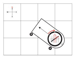
3. Hold compass level at waist height and turn yourself until the needle and orienting arrow are aligned. NOTE: Compensate for declination. See section 5.
