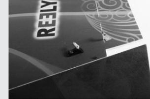
7. Pass the servo wire from the front through the carbon hole.
