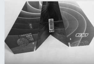
The back side carbon rod should be assembled into the slot. After determining the position, glue the bottom of the square carbon rod and the inside of the slot.
