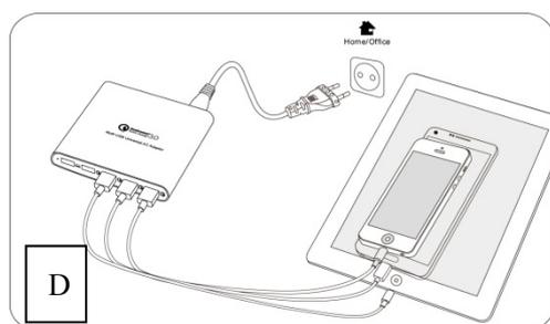
**Caution:** This adapter supports power 80W max. If your used power exceeds 80W, the adapter will occur to be over-load protection. When you re-plug the connection, then it will recover to normal work.
