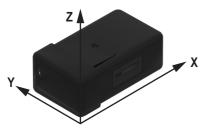
The following command sets the threshold of a position change to <slope threshold>. At the time, the current position in space is saved as a reference value. If the position deviates from the set reference value by the set threshold, an alarm is triggered.
