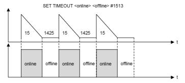
A sensor alarm or push on the external button "S1" will wake up the module at once.
