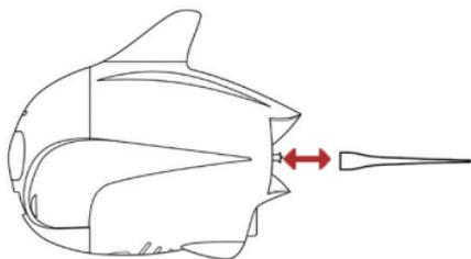
1. Hold the tail in horizontal direction and fix it to BIKI
