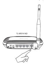
Launch the configuration utility and click WPS in the tools section. Select Push the button on my access point or wireless router and then click Connect.
