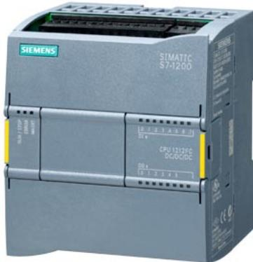
SIMATIC S7-1200F, CPU 1212 FC, Kompakt-CPU, DC/DC/DC, onboard I/O: 8 DI DC 24V; 6 DO 24V DC; 2 AI 0-10V DC, Stromversorgung: DC 20,4-28,8V DC, Programm-/Datenspeicher 100 KB
