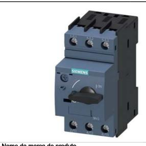
CIRCUIT-BREAKER SZ S00, FOR MOTOR PROTECTION, CLASS 10, A-RELEASE 10...16A, N-RELEASE 208A, SCREW CONNECTION, STANDARD SW. CAPACITY
