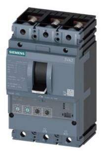
circuit breaker 3VA2 IEC frame 250 breaking capacity class H Icu=85kA @ 415V 3-pole, line protection ETU350, LSI, In=250A overload protection Ir=100A...250A short-circuit protection Isd=1.5...10 x Ir, Ii=10 x In nut keeper kit shunt trip (STL) 12-30V DC, 24V AC 50/60Hz
