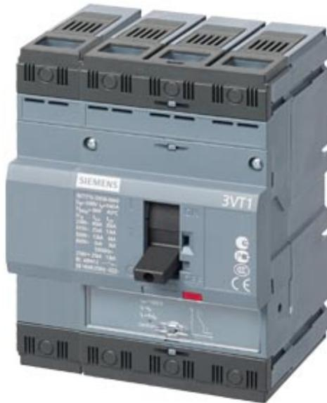
circuit breaker 3VT1 standard breaking capacity  $I_{cu}=25kA$ , 415V AC 4-pole, line protection trip unit TM,  $I_n=25A$  rated current  $IR=20...25A$  overload protection  $I=250...375A$ , short-circuit protection N conductor unprotected without auxiliary release without auxiliary/alarm switch with front terminals
