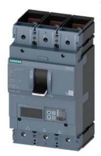
circuit breaker 3VA2 IEC frame 630 breaking capacity class H Icu=85kA @ 415V 3-pole, line protection ETU560, LSIG, In=630A overload protection Ir=250A...630A short-circuit protection Isd=0.6..9 x In, Ii=1.5..9 x In N conductor protection optionally with external current transformer, up to 160% gr.-fault prot., can be sw. off Ig=0.2...1 x In, tg=0.05-0.8s nut keeper kit undervoltage release (UVR) 208-230V AC 50/60Hz 2 auxiliary switches HQ
