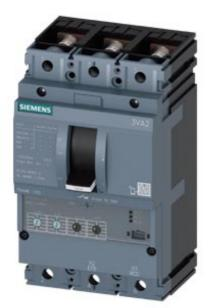
circuit breaker 3VA2 IEC frame 160 breaking capacity class M lcu=55kA @ 415V 3-pole, line protection ETU350, LSI, In=100A overload protection Ir=40A...100A short-circuit protection Isd=1.5...10 x Ir, li=12 x In nut keeper kit undervoltage release (UVR) 120-127V AC 50/60Hz
