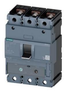
circuit breaker 3VA1 IEC frame 250 breaking capacity class M lcu=55kA @ 415V 3-pole, line protection TM240, ATAM, ln=160A overload protection Ir=112A...160A short-circuit protection Ii=5...10 x In nut keeper kit undervoltage release (UVR) 24V DC
