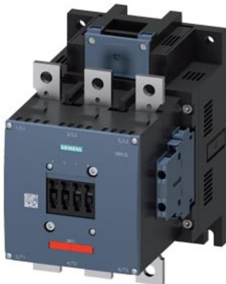
Power contactor, AC-3 225 A, 110 kW / 400 V AC (50-60 Hz) / DC operation 23-26 V UC Auxiliary contacts 2 NO + 2 NC 3-pole, Size S10 Busbar connections Drive: conventional screw terminal Auxiliary switch block 2 NO + 2 NC lateral, left + right Captive auxiliary switch, DIN 50012
