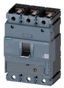
circuit breaker 3VA1 IEC frame 250 breaking capacity class H Icu=70kA @ 415V 3-pole, starter protection TM120M, AM, In=200A without overload protection short-circuit protection Ii=6...14 x In nut keeper kit shunt trip (STL) 12-30 V DC; 24 V AC 50/60 Hz 2 auxiliary switches HQ 1 trip alarm switch HQ
