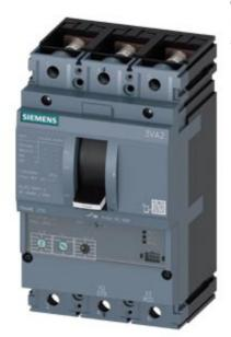
circuit breaker 3VA2 IEC frame 250 breaking capacity class C lcu=110kA @ 415V 3-pole, motor protection ETU350M, LSI, In=200A overload protection Ir=80A...200A short-circuit protection Isd=3...15 x Ir, Ii=15 x In nut keeper kit undervoltage release (UVR) 208-230V AC 50/60Hz 2 auxiliary switches HQ 1 trip alarm switch HQ
