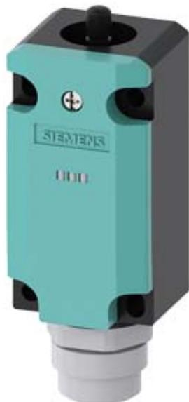
Basic switch for position switch 3SE51 Metal enclosure 40 mm according to EN 50041 with connector 6+PE according to EN 43651 with 2 LEDs, yellow/green 24 V DC 1 NO/1 NC slow-action contacts without actuator head Pin assignment: Pin1=21, Pin2=22 Pin3=14 and LED green, Pin4=13 and LED yellow, Pin5=not connected, Pin6=ground LED
