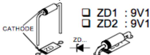
2. DIODE; PAZITE NA PRAVILNO POLARITETO!
