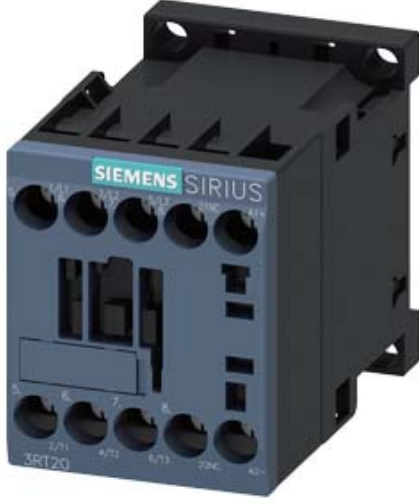
CONTACTOR, AC-3, 3KW/400V, 1NC, DC 24V, 3-POLE, SZ S00 SCREW TERMINAL
